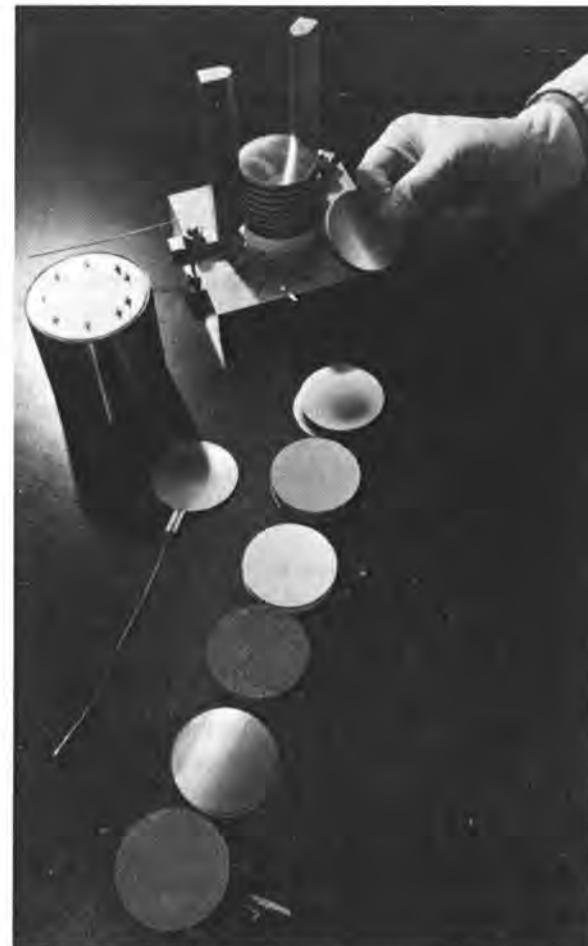
THERMAL BATTERIES are composed of poker-chip-like "pelletized cells." Activated by heat, modern thermal batteries contain no liquids and, once packaged in a metal cylinder (upper left), are rugged, long-lived, and reliable.
